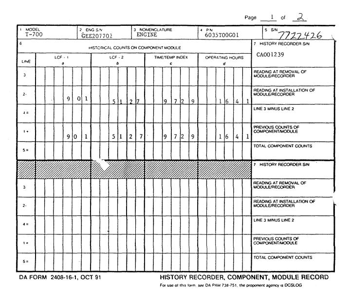
Figure 13. Sample of a completed DA Form 2408-16-1 (History Recorder, Component, Module Record (Engine showing major modules and components)). (Sheet 1 of 3)
