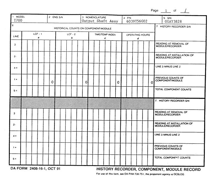
Figure 14. Sample of a completed DA Form 2408-16-1 (History Recorder, Component, Module Record (on new engines, components or modules for spares). (Sheet 1 of 2)
